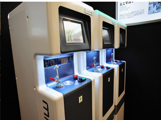
図 7 Minimal fabrication of semi-conductor
