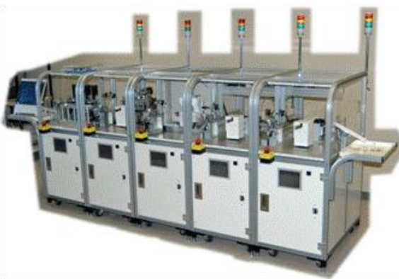
図3 Compact modular production system for MEMS device
